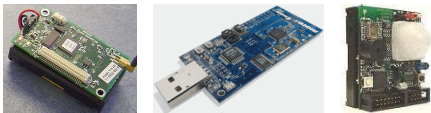
Fig. 2. Current sensor node hardware: Mica 2 by Crossbow, Berkeley (from [15]); Tmote sky by moteiv, Berkeley (from [20]); and Embedded Sensor Board by Scatter-Web, Berlin (from [5])
